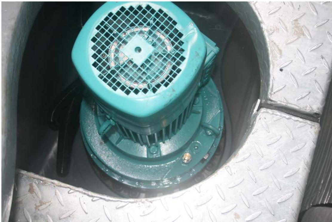
Figure 20 Left front yaw drive mounted on bedplate viewed through catwalk cutout.
