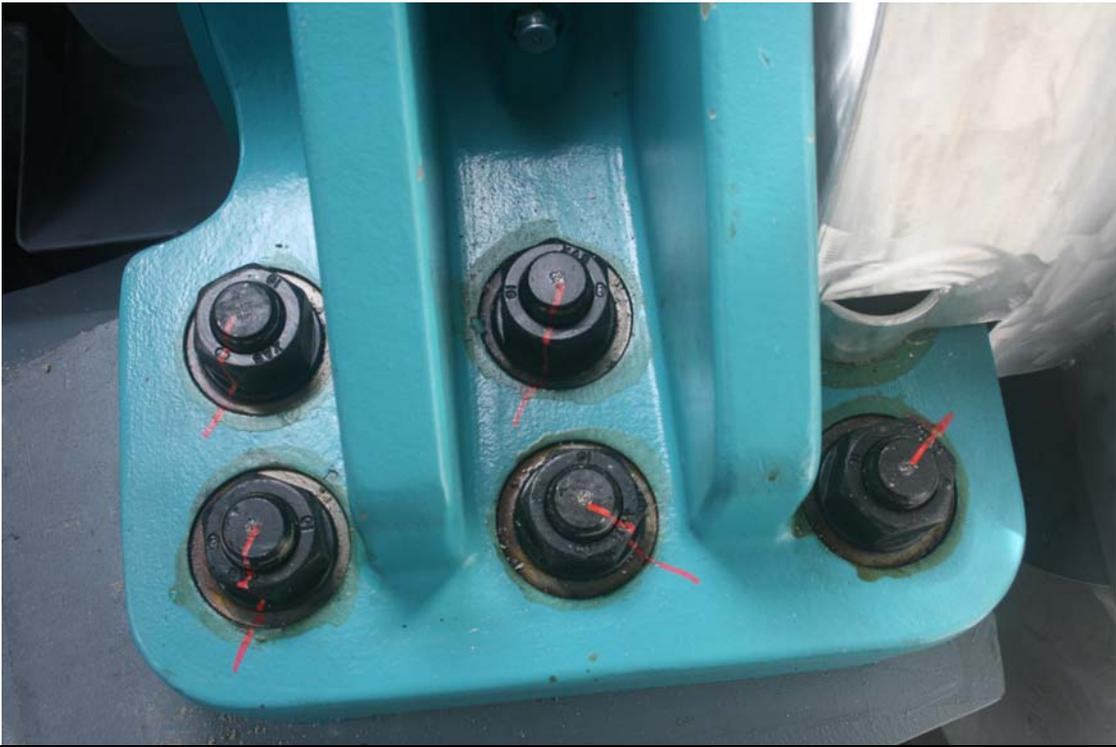
Figure 51 Main pillow block bearing right side bolting.
