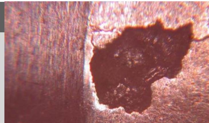
**SKF:** “...damaging effects of stray bearing currents include increased noise and heat levels, reduced effectiveness of the lubricant, excessive vibration and eventually, premature bearing failure.”
